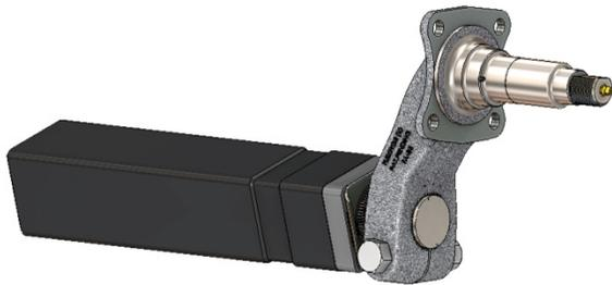
*The **Flexiride**® rubber torsion axle consists of three primary components: a rubber cartridge, support bushing and spindle arm. The cartridge is comprised of strong proprietary formula rubber bonded to a steel shaft.*
